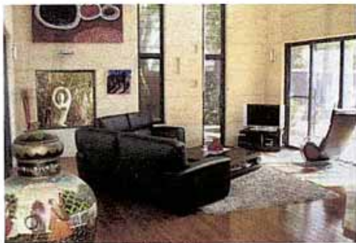
Rammed-earth walls in the living area are attractive and control the temperature range inside all year.
